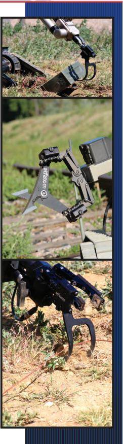
Users can easily interchange tools via Picatinny Rails and an innovative gripper mounting method.
